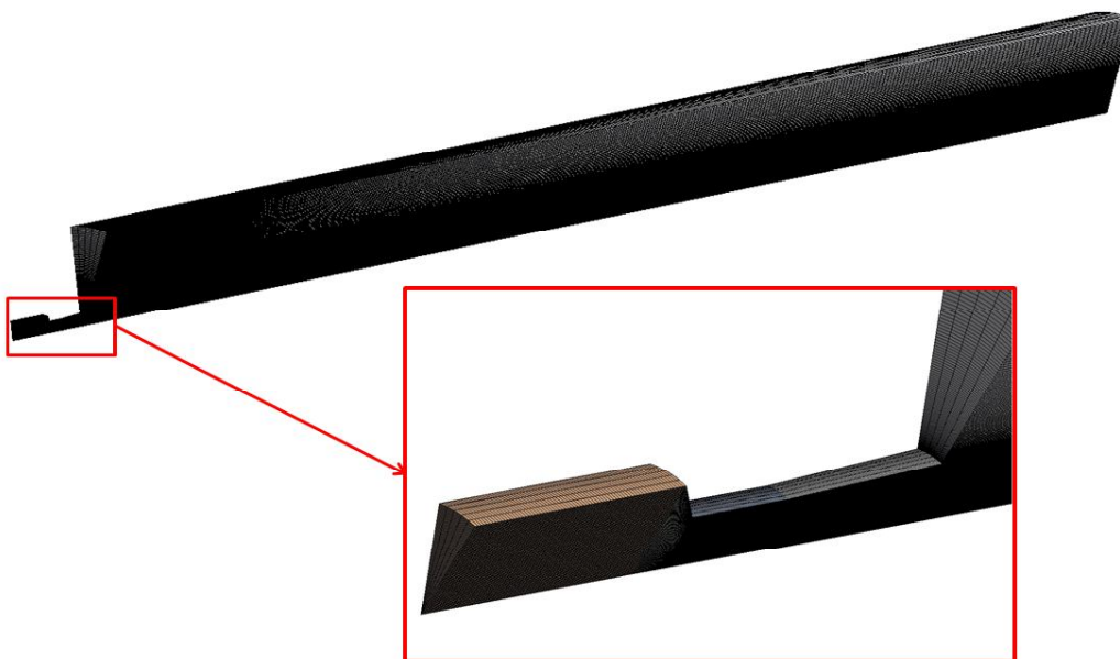
Figure 7: Mesh used in CFD simulation composed for 1.500.000 hexahedral elements.
