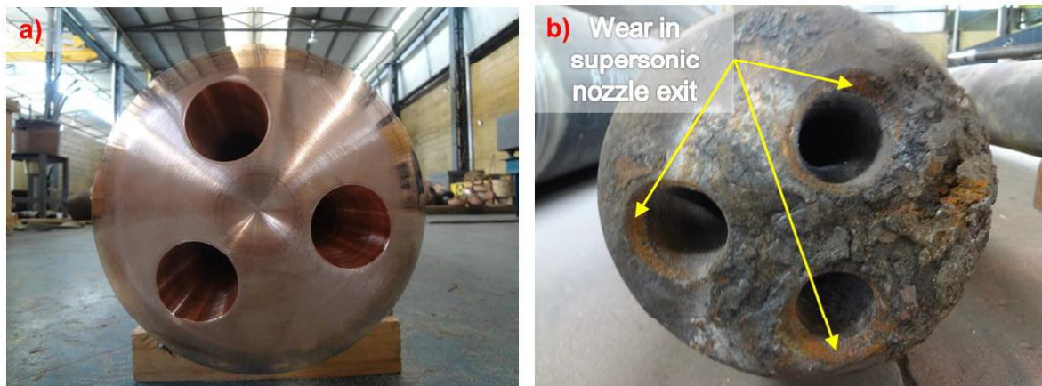
Figure 4: a) New tip; and b) Same tip after 600 heats, displaying nozzle wear.
